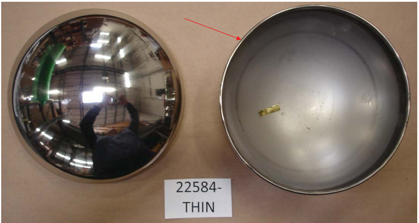
P/N 22584-THIN – IS A THIN LIP – LOOK WHERE THE ARROW IS POINTING. THIS IS THE 8 1/4"
